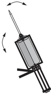
Hold cartridge upward and load into gun.
